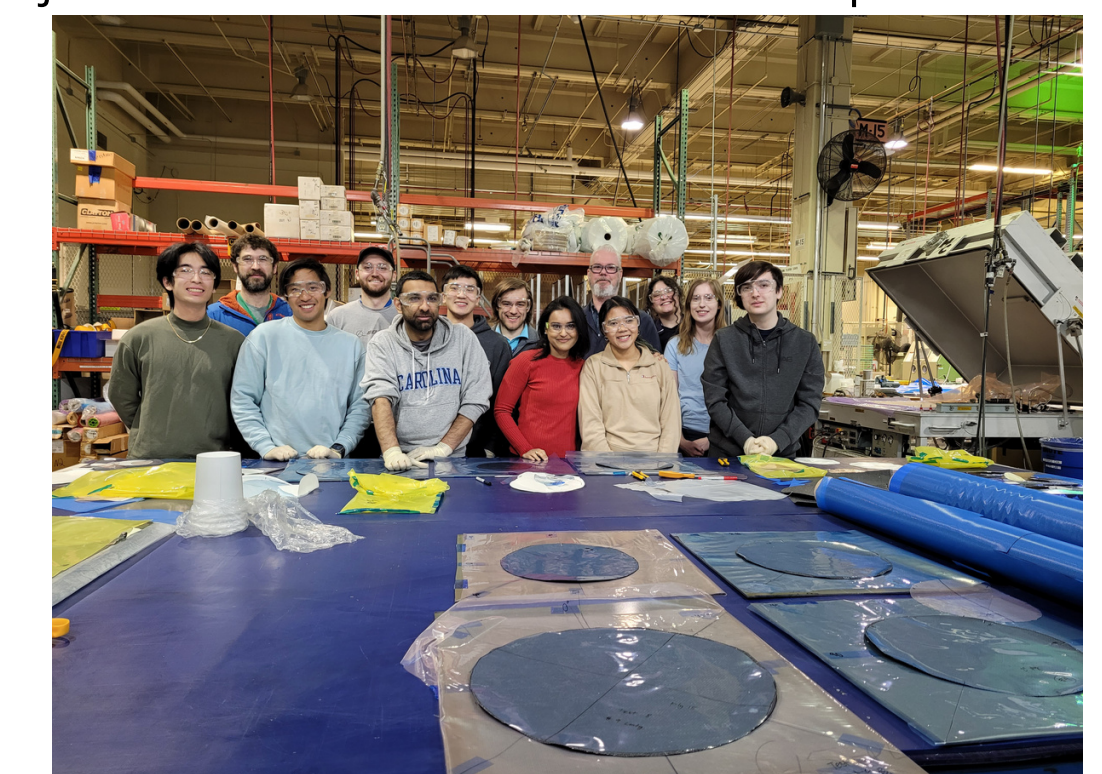
Figure . Students and Boeing mentors at John Spalding's lab with scarfed panels ready for double vacuum debulk.
